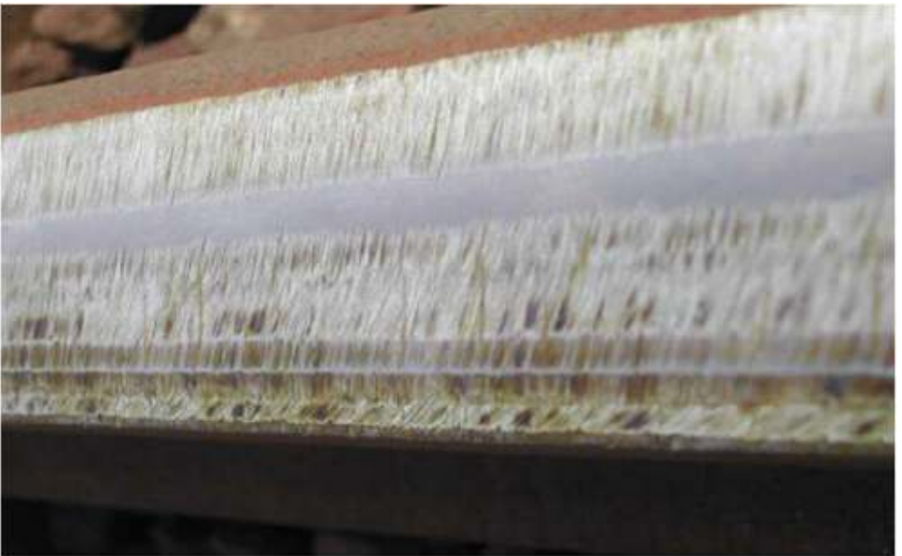
Fig. 8.42 - Poor surface finish after grinding – skipped grinding
