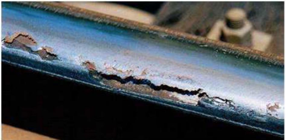
Fig. 8.10 - Very severe shelling
