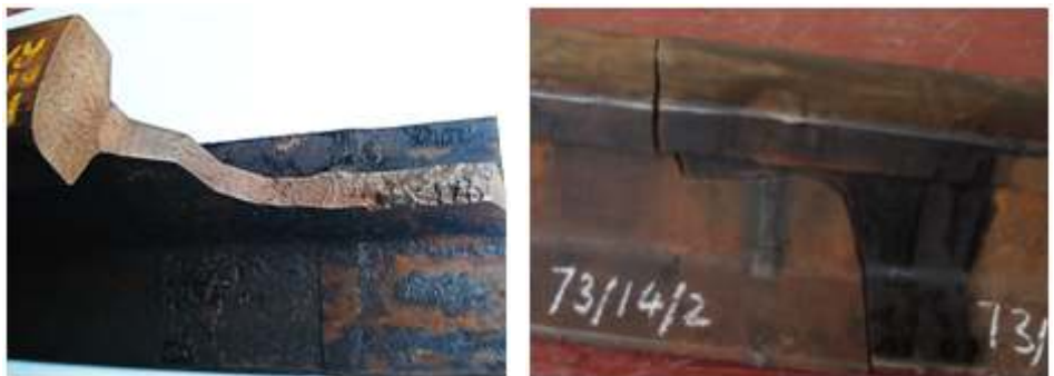
Fig. 8.26 - Welding, flash butt joint, horizontal crack
