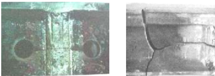
Fig. 8.28 - Welding, thermit joint horizontal crack
