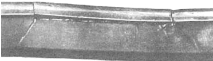
Fig. 8.17 (b) Head web junction at top fillet radius.
