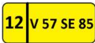
Fig. 5.09 Template showing station, versine and super elevation.
