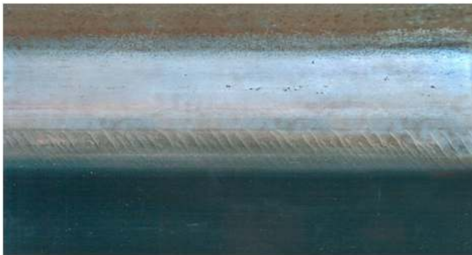
Fig. 8.07 – Gauge corner cracks
