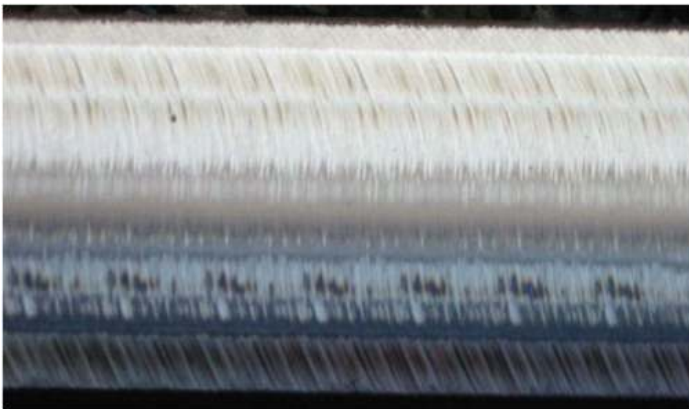
Fig. 8.43 - Skipped grinding & blueing of rail
