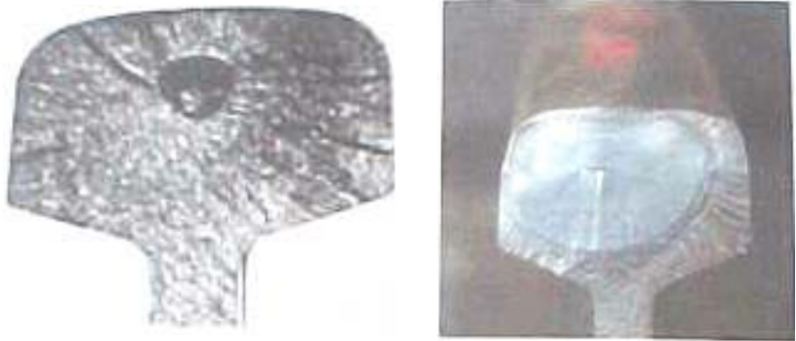
Fig. 8.22 - Transverse fatigue crack in head
